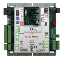
Advanced Application Controller (AAC) designed for controlling a single zone in a building. The ZN551 is well suited for VAV, heat pump, unit ventilator and other packaged HVAC applications. It communicates on an EIA-485 LAN using BACnet MS/TP or BACnet over ARCNET communications and connects seamlessly to the WebCTRL® building automation system.
